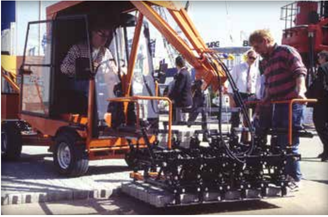
Figure 3. Motorized equipment with a mechanical clamp.
