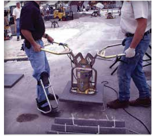
Figure 21. Vacuum assisted mechanical equipment for installing paving slabs.
