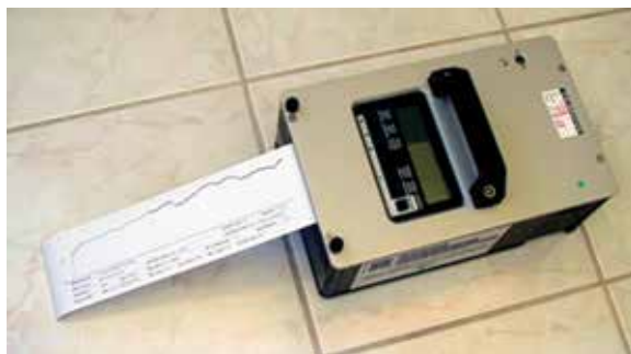
Figure 2. The BOT 3000 device measures the dynamic coefficient of friction (DCoF) and is manufactured by Regan Scientific Instruments, Inc., in Southlake, Texas. Photo credit: Jack Trumpet
