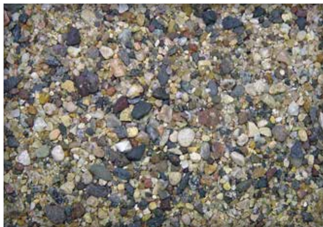
Figure 3. Example of sand from the ICPI bedding sand test program with a total combined percentage of sub-angular and sub-rounded particles equal to 65% according to ASTM D2488
